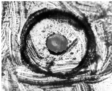
Figure 7-6. Damage from improper cleaning.
